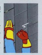
hooks the base of the slate Slide new slate into place Then gently pull the hook pull until the Hallhook™ Do not over stretch Remove hook pull.
