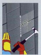
Position Hallhook™ between slates so that bottom hook slate baseline and fix with is 10mm above finished nail. Hang hook pull on Hallhook
